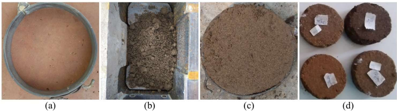
Figure 3. (a) The cylindrical metallic mould for making the compressed earth block samples; (b) The mould placed inside the normal brick mould; (c) The wet compressed earth block that was still inside the cylindrical mould; (d) Some of the prepared compressed earth block samples.
