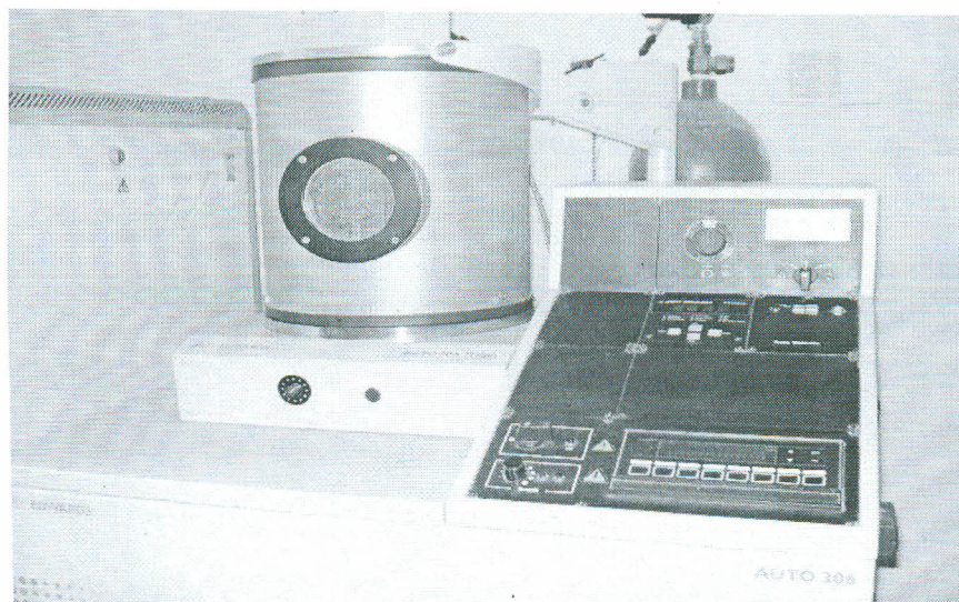
Fig 4.1: Edwards Auto 306 coating unit.
