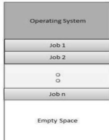
Figure 4.11: Memory Layout in single processor system (Source: Research)
